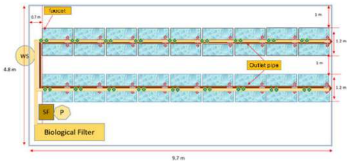
Fig 8: Layout of the larva rearing unit (Unit A) with 36 aquariums. SF: Sand filter; WP: water pump, WS: Water storage. Red line: filtered water flow to the tank, yellow line: wastewater from the aquarium. The wastewater flows (yellow line) into the biological filter by gravity and enters the biological filter and sand filter; then drawn by a pump, which directs it a sand filter before entering the storage tank. Water from the storage tank is distributed to all aquariums.
