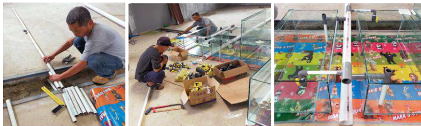
Fig 14: Preparation of inlet and outlet pipe components for aquariums
